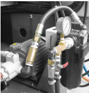
Basic supply unit for IKZ (internal coolant supply), 18 bar
