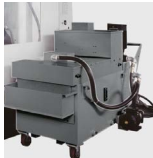
Belt filter unit on cooling water tank
